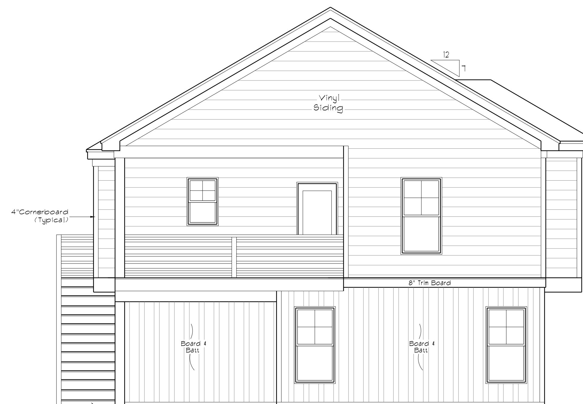
Rear Elevation Scale: 1/4" = 1'-0"
